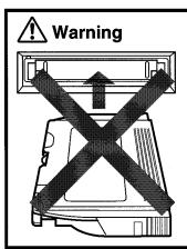
Be careful to insert the cartridge the correct way round. If inserted sideways, it can damage the read/write head.
